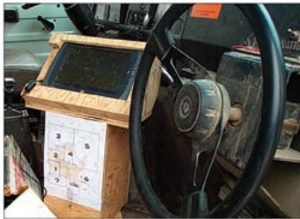
Computer mounted on pedestal inside recycling truck
